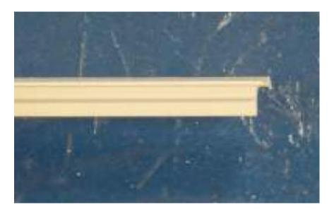
5.) Clean the weld corners at the ends to allow the notched portion of the mull cover to sit flat and flush when snapped in place.
